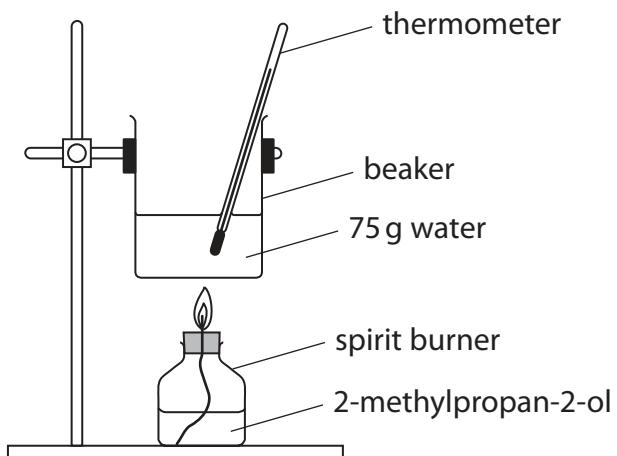
A sample of 2-methylpropan-2-ol was burned in a spirit burner and used to heat 75 g of water. The results are shown.
